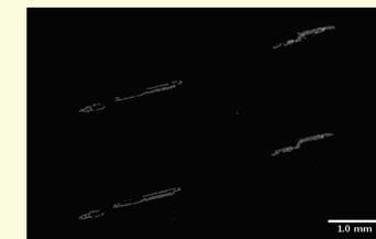
Figure 7: A thresholded version of Figure 6. Each pixel is designated with a grayscale intensity as background, ice, or brine leading to the image above.
