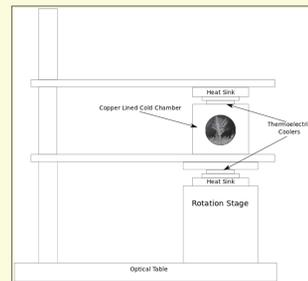
Figure 2: Schematic of the cold stage used to control sample temperature. The cold chamber and Peltier coolers are encased in foam (omitted in schematic for clarity).
