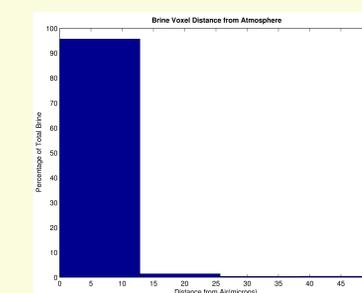
Figure 8: The above plot shows the percentage of brine within certain distances of the surface. The bar width is set using the voxel size of the data set, in this case 12.84 microns. The brine to air distance is calculated by analyzing a sub-volume of increasing size centered on each brine voxel.
