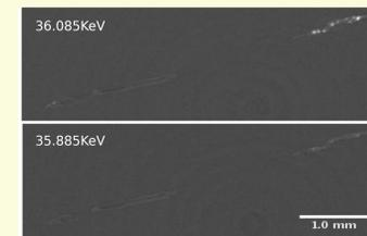
Figure 6: One slice imaged at differing X-ray energies shows the increased absorption of Cs as the increased X-Ray energy causes excitation of K shell electrons.
