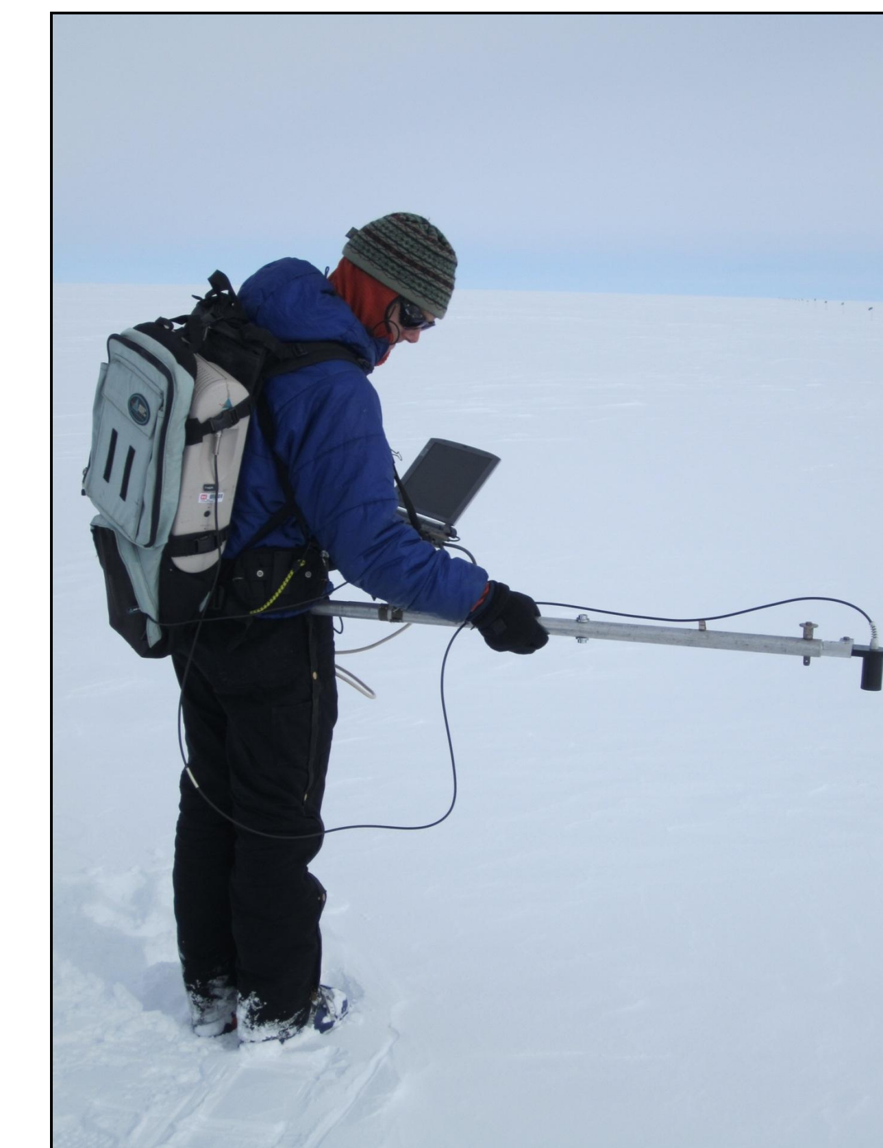
Fig. 4. Taking an upwelling measurement with the ASD FieldSpec Pro at Summit, May, 2011.
