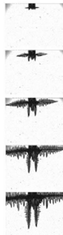
Dendrite formation in Li/polymer batteries for electric vehicles
